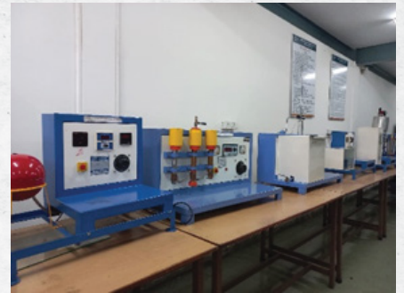
Advance heat pipe performance test rig
