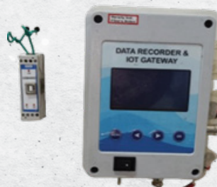
Dual channel solar PV VI characteristic logger
