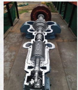
Turbine Generator set full scale model
